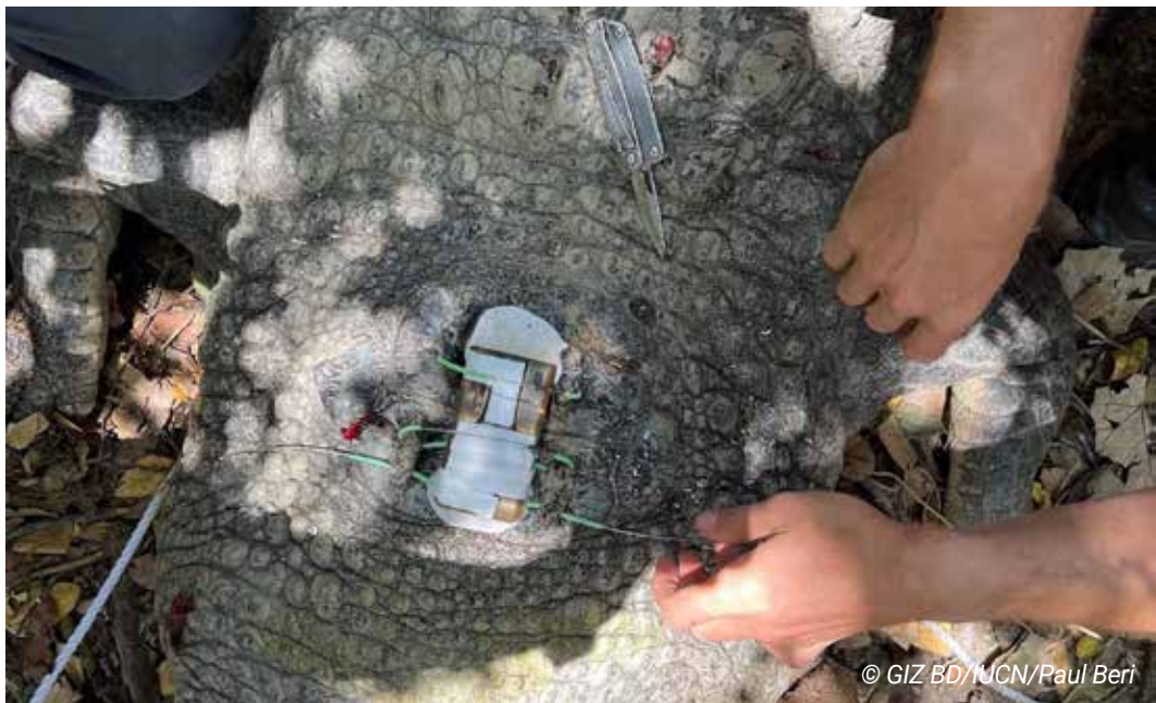
A tag being attached to the nuchal shields of a large Saltwater Crocodile. Note the tape covering the sensors and lumo tubes added to the trace wire that goes through the holes drilled in the scutes.
